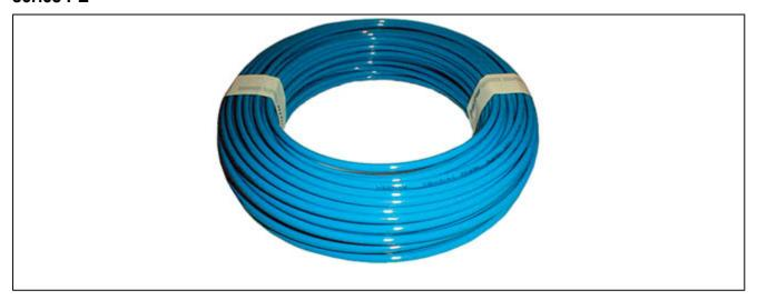
basic material polyethylene, recyclable -10°C to +60°C temperature range vacuum -0,87bar to values in table at 30°C, pressure reduction factors see table operating pressure tolerance of outside diameter ±0,10mm tolerance material thickness ±0,10mm length of rolls 50m colours normally blue, yellow, green, natural, black application compressed air uses, control pipes in laboratory techniques and apparatus engineering
